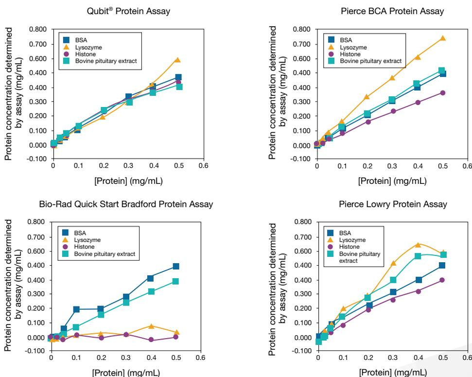
**Figure 4. Protein-to-protein variability.** Triplicate samples of BSA, lysozyme, histone, and bovine pituitary extract were assayed at concentrations of 0–0.5 mg/mL using the Qubit® Protein Assay on the Qubit® 2.0 Fluorometer, and various other protein quantitation methods. The variability at 0.3 mg/mL for the Qubit® assay was found to be <7%.
